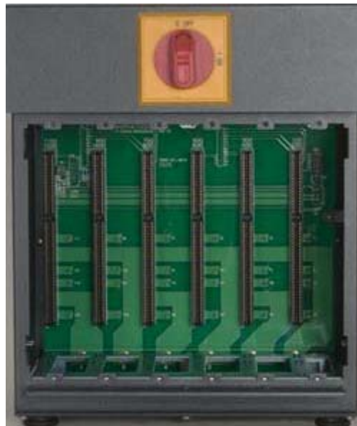
Mainframe Bay with Backplane Exposed
