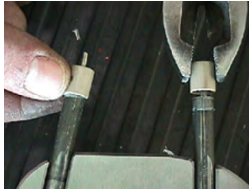
Figure 6-120: PEEK Bushing Removal and Installation
