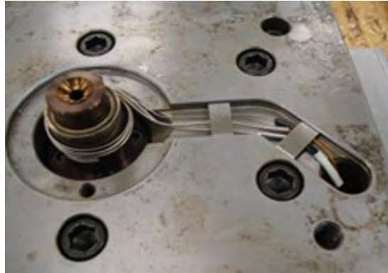
Figure 6-118: Wire Wrapped Around Sprue Heater
