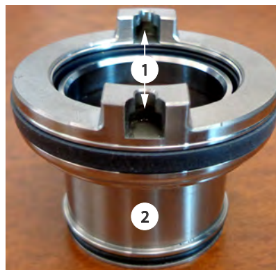
Figure 4-25: Cylinder Insert and Annular Piston Assembly
