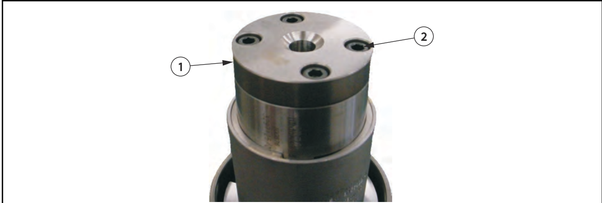
Figure 4-39: Sprue Bushing Insert Installed
