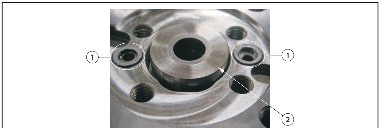
Figure 4-46: Grafoil Seals and M-C Reducer in Air Plate
