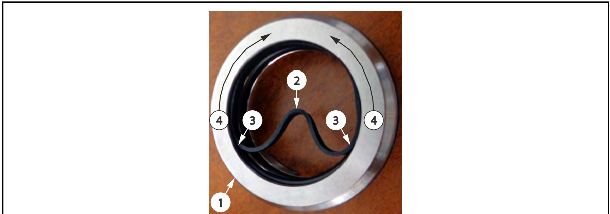
Figure 4-19: Installing the Inner Double Delta Seal Ring
