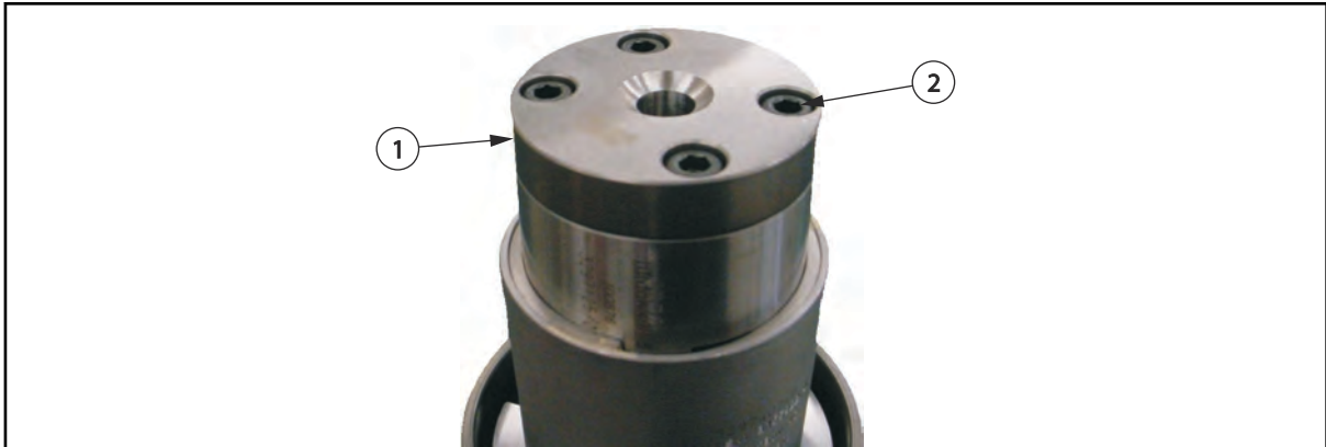
Figure 4-73: Sprue Bushing Insert Installed
