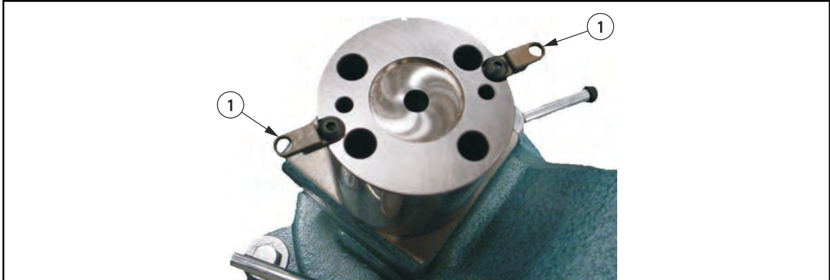
Figure 4-47: Sprue Body Retaining Tabs
