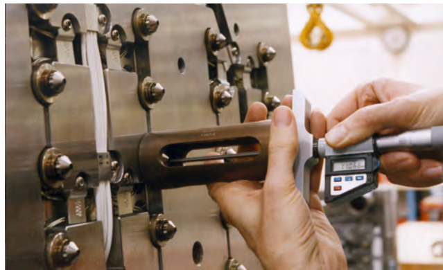
Figure 6-12: Measuring the Nozzle Tip Height
