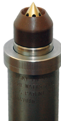
Figure 6-57: Seating the Nozzle Tip Insulator (Example)
