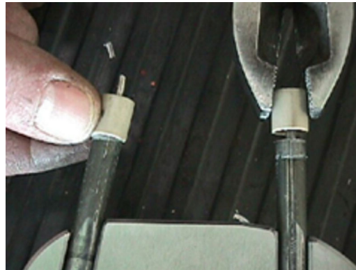
Figure 6-67: PEEK Bushing Removal and Installation
