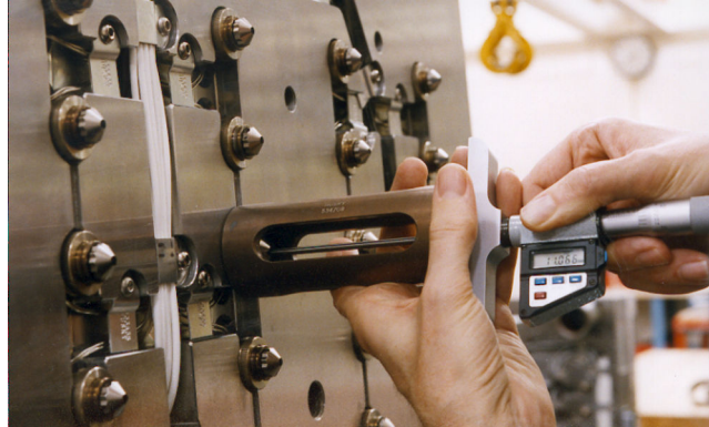
Figure 6-64: Measuring the Nozzle Tip Height
