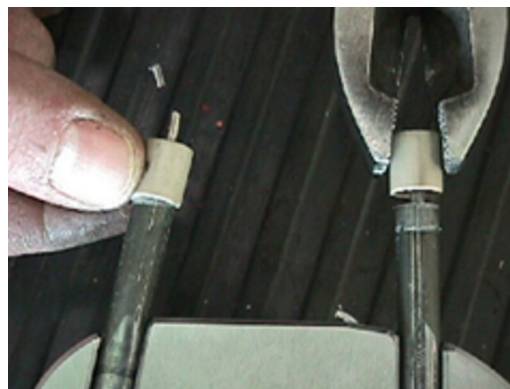
Figure 6-118: PEEK Bushing Removal and Installation
