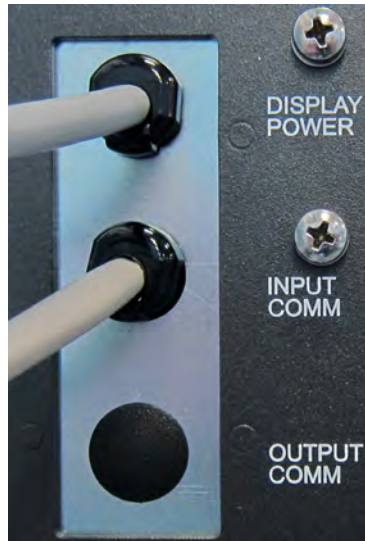
Figure 2-17 Display Power and Temperature Control Connections
